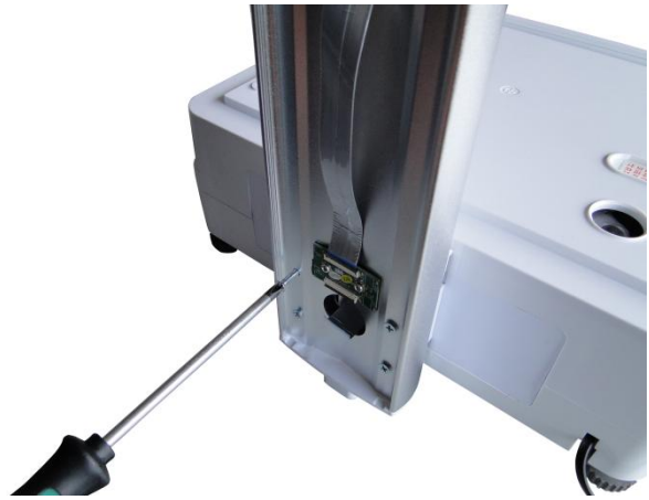
3 Screw the screws as circled in the picture and wind the line of the machine to front through display pole rod.
